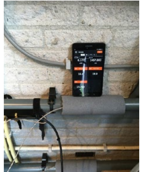
The PT900 programmed for energy measurement
