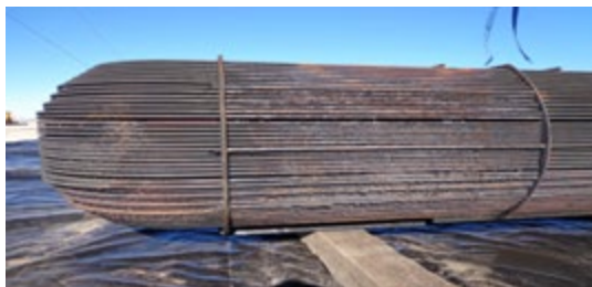
Salt corrosion and fouling was reduced after 18 months with TOPGUARD 1130 salt control additive
