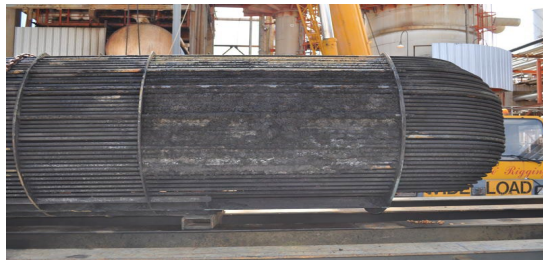
Salt corrosion and fouling after only eight months with traditional treatment program
