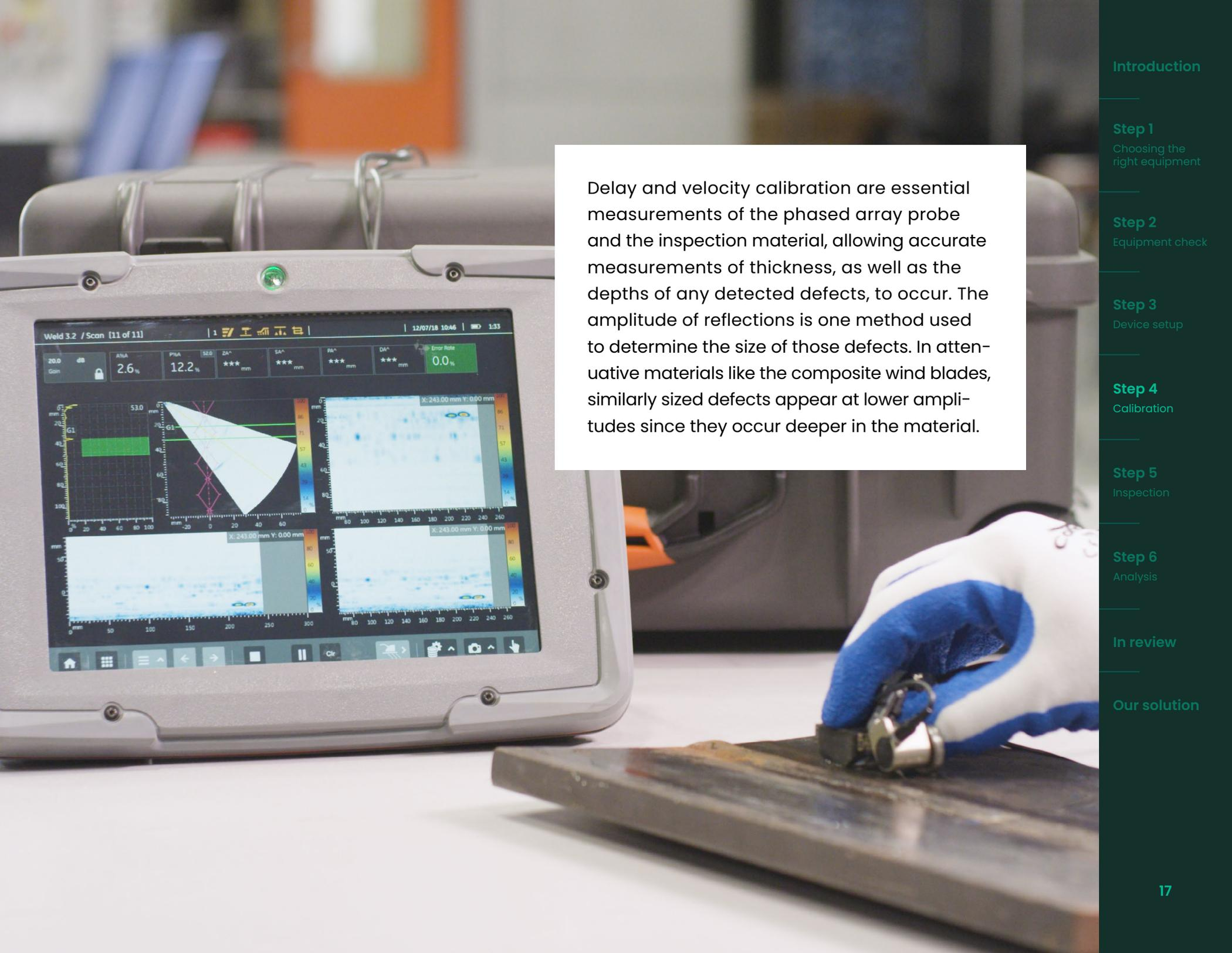
Delay and velocity calibration are essential measurements of the phased array probe and the inspection material, allowing accurate measurements of thickness, as well as the depths of any detected defects, to occur. The amplitude of reflections is one method used to determine the size of those defects. In attenuative materials like the composite wind blades, similarly sized defects appear at lower amplitudes since they occur deeper in the material.
