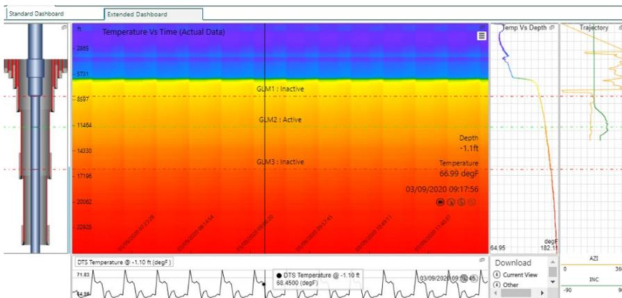
The ProductionLink DTS dashboard provides an overview of temperature data in 2D and gas-lift mandrels along with the line markers.
