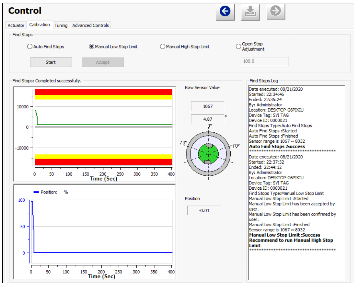
Figure 53 - Manual Low Stop Limits Results: Succeeded
