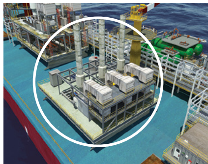
Intermediate-Pressure Gas-Lift Compressors
