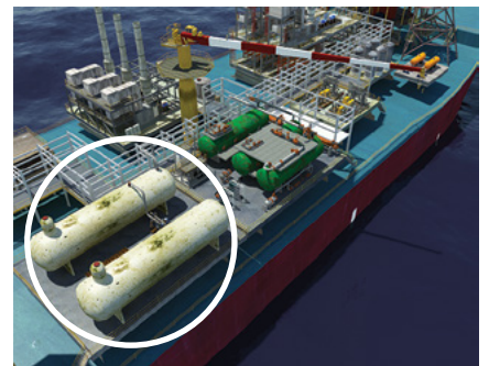
Crude Oil Treatment, Desalting
