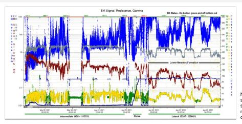
NaviTrak UT's post-run software displays EM signal strength, resistance, and gamma across the entire well
