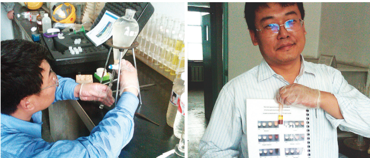
The LeakID test is a proprietary investigative tool used by Baker Hughes engineers to identify and quantify the type of hydrocarbon leaks in cooling water systems. The refinery had several possible locations for benzene leaks.
