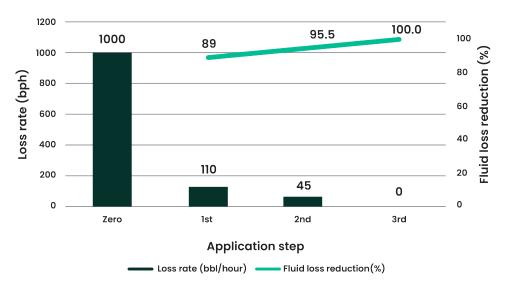
The three-stage SOLU-SQUEEZ displacement dramatically reduced fluid losses after just the first pill and resulted in the complete curing of losses after the third pill.
