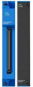
The Protection Processing Module (PPM) serves as the computational engine for the Orbit 60 monitoring system. It extracts all machinery measurements for the protection system and performs alarm determinations. The PPM analyzes signals from transducers, generates measurements and statuses and publishes them to other modules for data collection and external communication. Each PPM occupies a single slot within the system.
