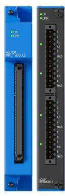
The Orbit 60 Series AC LVDT Input Module provides inputs to interface with four AC Linear Variable Differential Transformers for position measurements. The module's primary use is the measurement of case expansion and valve position. The AC LVDT input module occupies a single slot.
