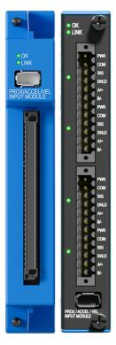
The primary purpose of the Dynamic Input module is to digitize the sensor signal at a rate that completely encompasses the signal content and provides transducer power for various sensors. The Orbit 60 Series Dynamic Input modules are a set of 4-channel input modules available in both negative and positive dynamic input options. The inputs are also used for speed or Keyphasor signals.
