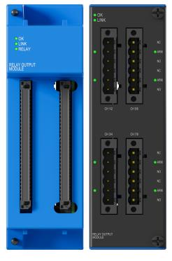
Relay modules may be programed to actuate based on alarm conditions defined in other modules. Use standard logic elements (True AND, Normal AND, OR and NOT) to combine various alarms and statuses (e.g. OK statuses, Bypass, Protection State, Inhibit, Attention, Protection Fault, etc.) into relay activation conditions. Orbit Studio is used to program the voting logic.
