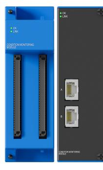
The Condition Monitoring Module (CMM) listens to all information within the system, including all measurements, waveforms, digital transducer signals, system controls, status information, system configuration information, process data from external systems, and alarm and events logs. It only listens, with no capability to write, allowing interface to System 1 over the business networks, with no risk to the protection system.
