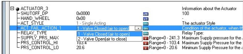
Figure 112 - Transducer Block - Fail Action Parameter
