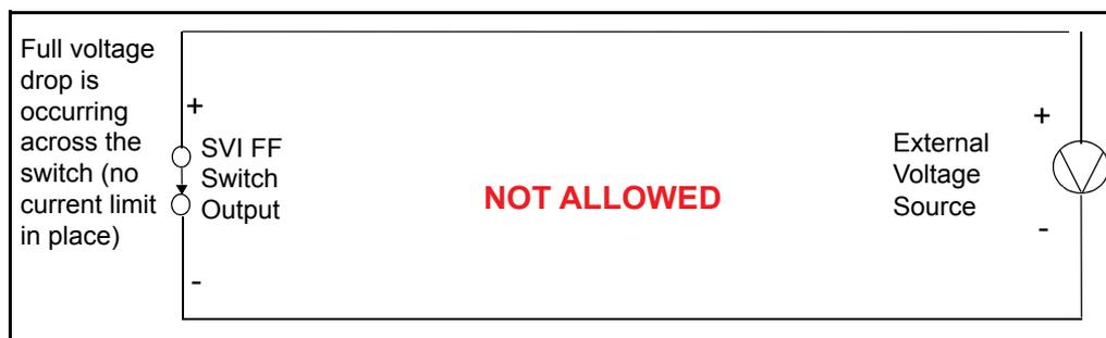
**Figure 34 - Switch Installation Drawing without Load: Configuration Not Allowed**
