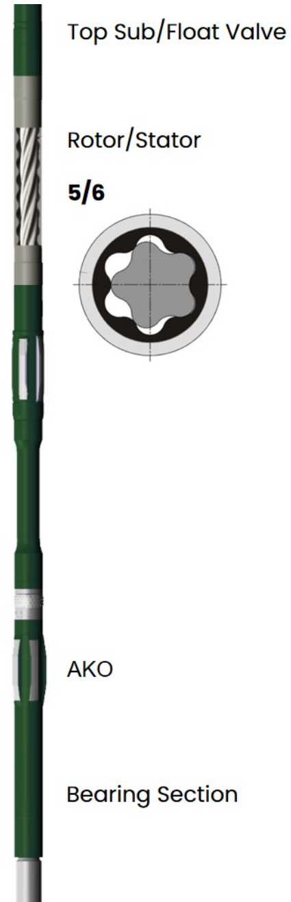
5 1 / 8 -in. Navi-Drill DuraMax D050-5065C Motor
