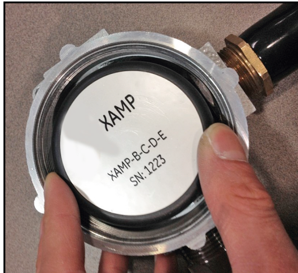
Figure 22: Junction Box Cap
