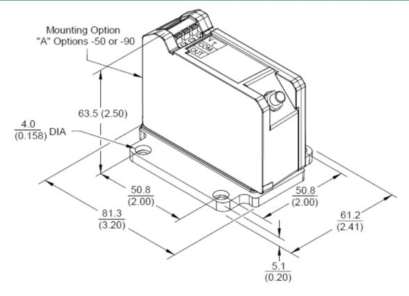
Figure 15: Panel Mount 3300 XL 11 mm ProximitorSensor
