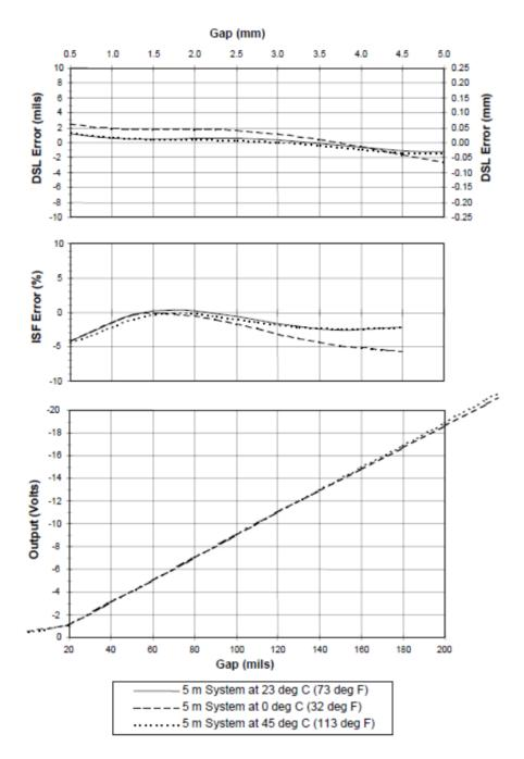
Figure 1: Typical 3300 XL 11 mm 5 m System Over Ambient Testing Range
