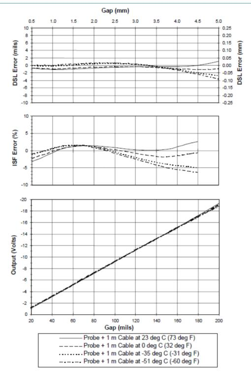
Figure 3: Typical 3300 XL 11 mm Probe + 1 m Cable @ Low Temperature
