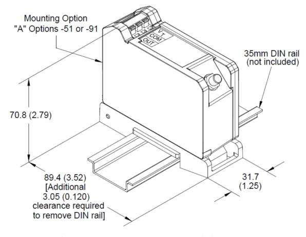
Figure 16: DIN Mount 3300 XL 11 mm Proximitor Sensor
