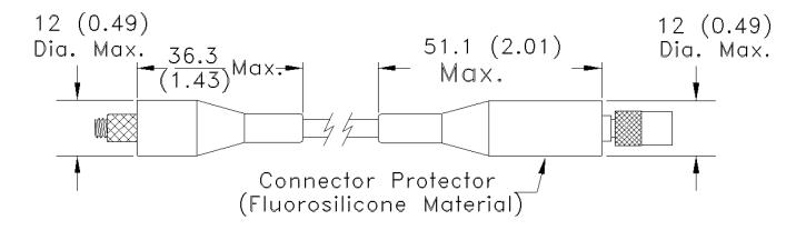
Note: Connector Protector only installed on female end when optioned. Both ends available as accessories.
