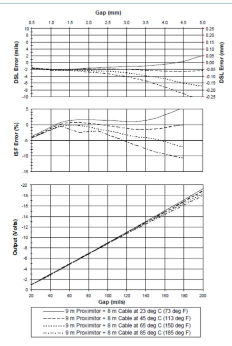
Figure 8: Typical 3300 XL 11 mm 9 m Proximitor with 8 m of Extension Cable @ High Temperature (Probe is at 25°C.)
