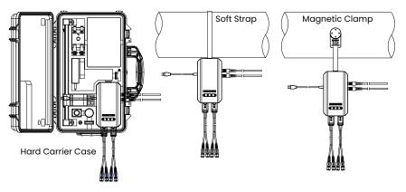
Figure 6: PT900 Transmitter Mounting Options
