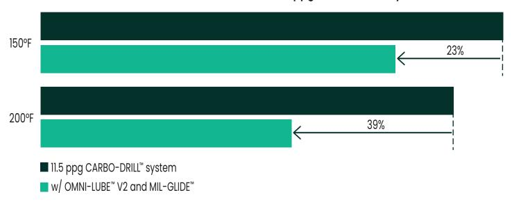
In HT/HP lubricity testing, the OMNI-LUBE V2/MIL-GLIDE formulation demonstrated superior lubricity and the greatest reduction in the coefficient of friction of any other fluid tested.
