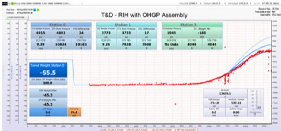
Real-time weight at service tool plotted against modeled data with differing friction factors
