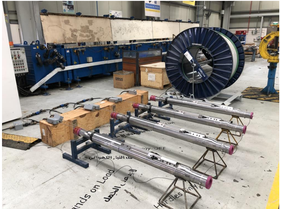
A system integration test (SIT) was conducted and all equipment and installation kits were inspected prior to mobilization and tested upon arrival to the rig site to ensure complete job readiness.
