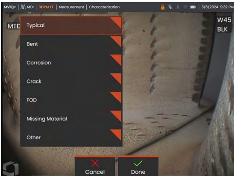
Drop-down classifications available on a VideoProbe running an MDI Template “Turbine”
