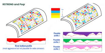
Difference between Psqr and RSTRENG – interacting corrosion in shape is more accurately characterized to avoid unnecessary repairs.
