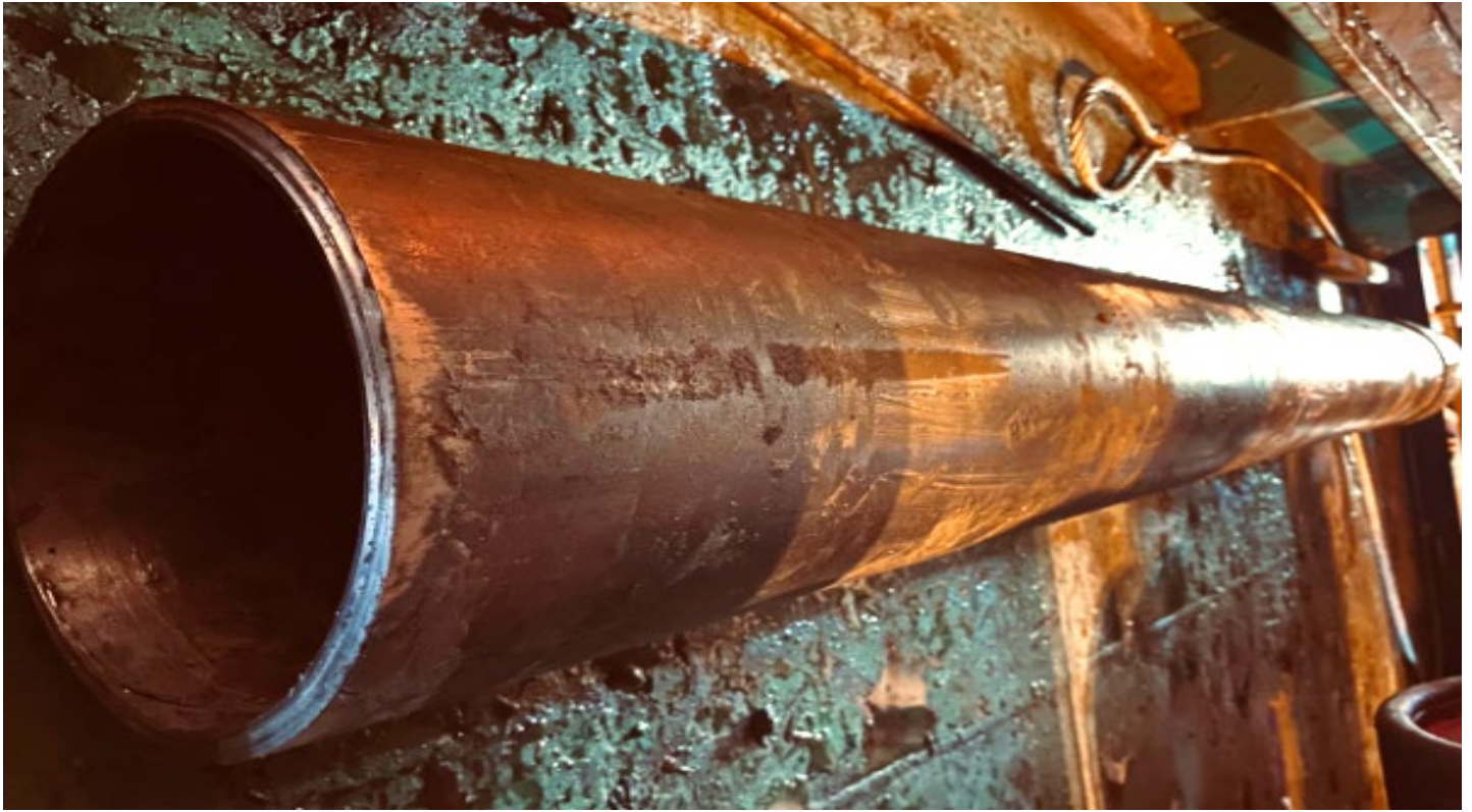
9 5/8-in. casing stump, with clean cut.
