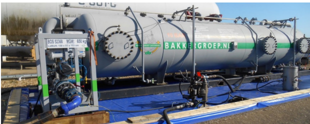
38,000 L separator complete with emergency shutdown valve (70% liquid level and 5.2 barg high-pressure ceiling) and large-diameter, pressure-regulating valves. Approximately 20,000 sm 3 of gas passed through this unit, removing over 400 m 3 of condensate and contaminated liquids
