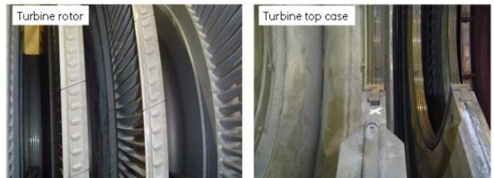
Figure 9: Signs of rub as seen from turbine rotor and top case
