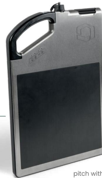
Ruggedized detector with 8 x 8" GOS scintillator, 200 µm pixel pitch with optimized imager design for excellent image quality, wide dynamic range and improved dose efficiency with both X-rays and Gamma-rays
