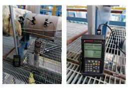
Panametrics originally recommended its BWT technology, but due to the premium alloys needed to manufacture a wetted flow meter, it exceeded the customer's budget. Panametrics subsequently recommended a clamp-on solution. However, the customer was not convinced the solution would be successful. Therefore, Panametrics carried out a trial on site to prove the technology.
