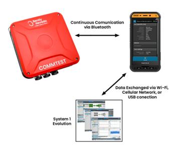
The COMMTEST portable connects via Bluetooth to the handheld, which you can then sync with System 1.
