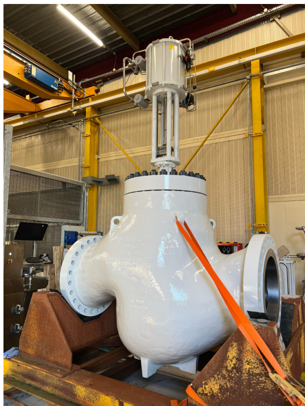
Figure 2. Compressor anti-surge control valves couple large capacity with precise, high-speed control.
