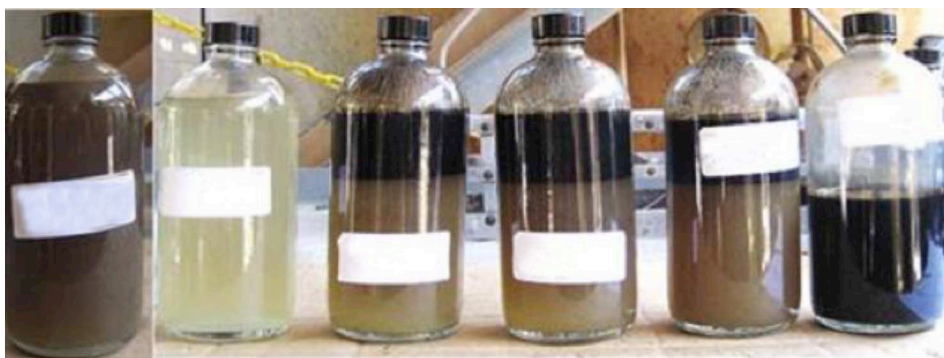
Fig 2 - B. Brine and Trylines 1 to 5 with XERIC treatment program after 4 hours, clear water at 17 in., oil-free brine with high solids (L-R)
