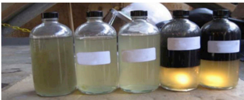
Fig 2 - C. Brine and Trylines 1 to 4 with XERIC treatment program, after 24 hours, clear water at 24 in., oil-free solids (L-R)
