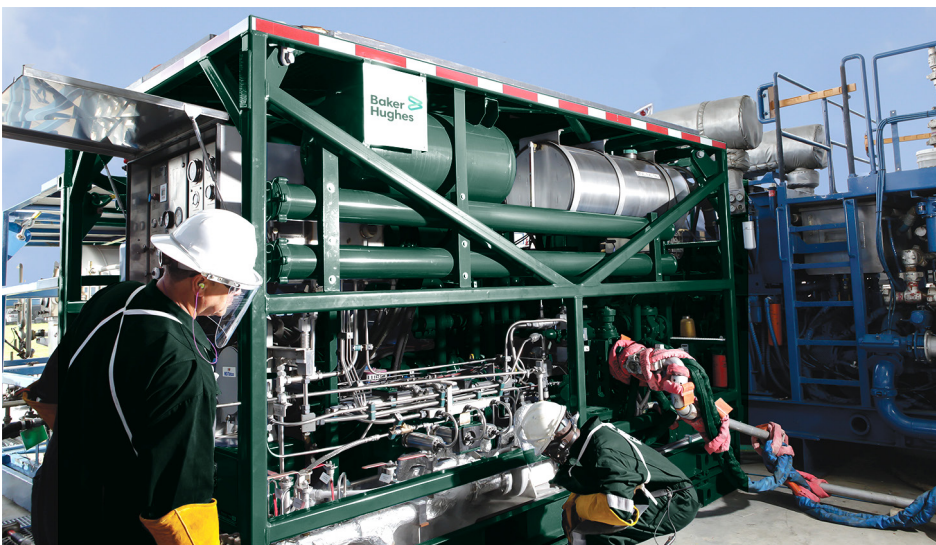
The Baker Hughes FoamSet liquid foaming system.
