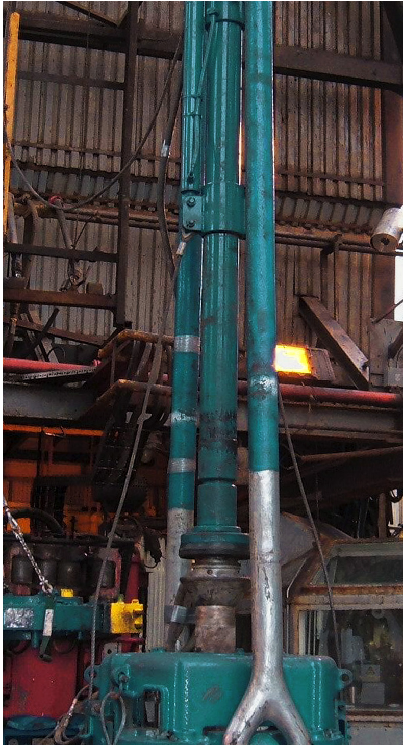
T-CAT tool showing the FAC tool partially inside the casing ready for fill-up operations, and the main elevator.
