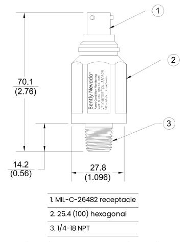
Figure 2: Dimensions for 330525 Velomitor XA Piezo-Sensor
