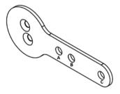
Figure 10 - Lever for Masoneilan Model 87/88 Multi-spring Actuator
