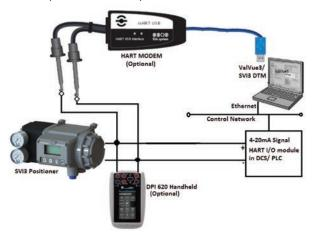
Figure 14 - Wiring Diagram
