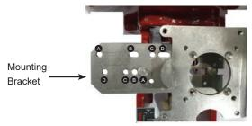
Figure 8 - Reciprocating Valve Mounting Bracket
