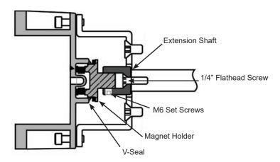
Figure 6 - Camflex V-Seal
