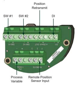
Figure 17 - Optional Modual Connections
