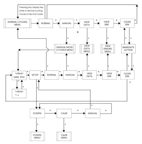
Figure 19 - Pushbutton Menu Structure
