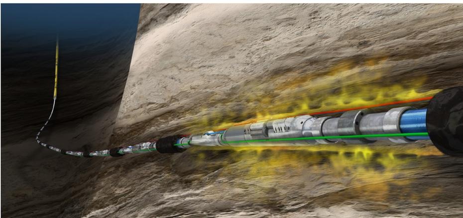
By installing a MultiNode all-electric intelligent completion system coupled with the SureVIEW DAS system, the operator can now remotely control and monitor water injection in all four individual zones. In addition, the intelligent completion provides the ability to continuously acquire, aggregate, transmit, store, process, analyze and visualize gigabytes of surveillance data from a variety of multi-sensors for real-time monitoring and optimization of the intelligent injection well operations.
