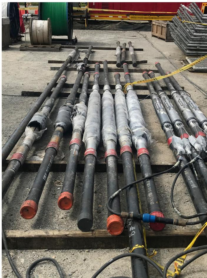
MultiNode equipment layout prior to installation
