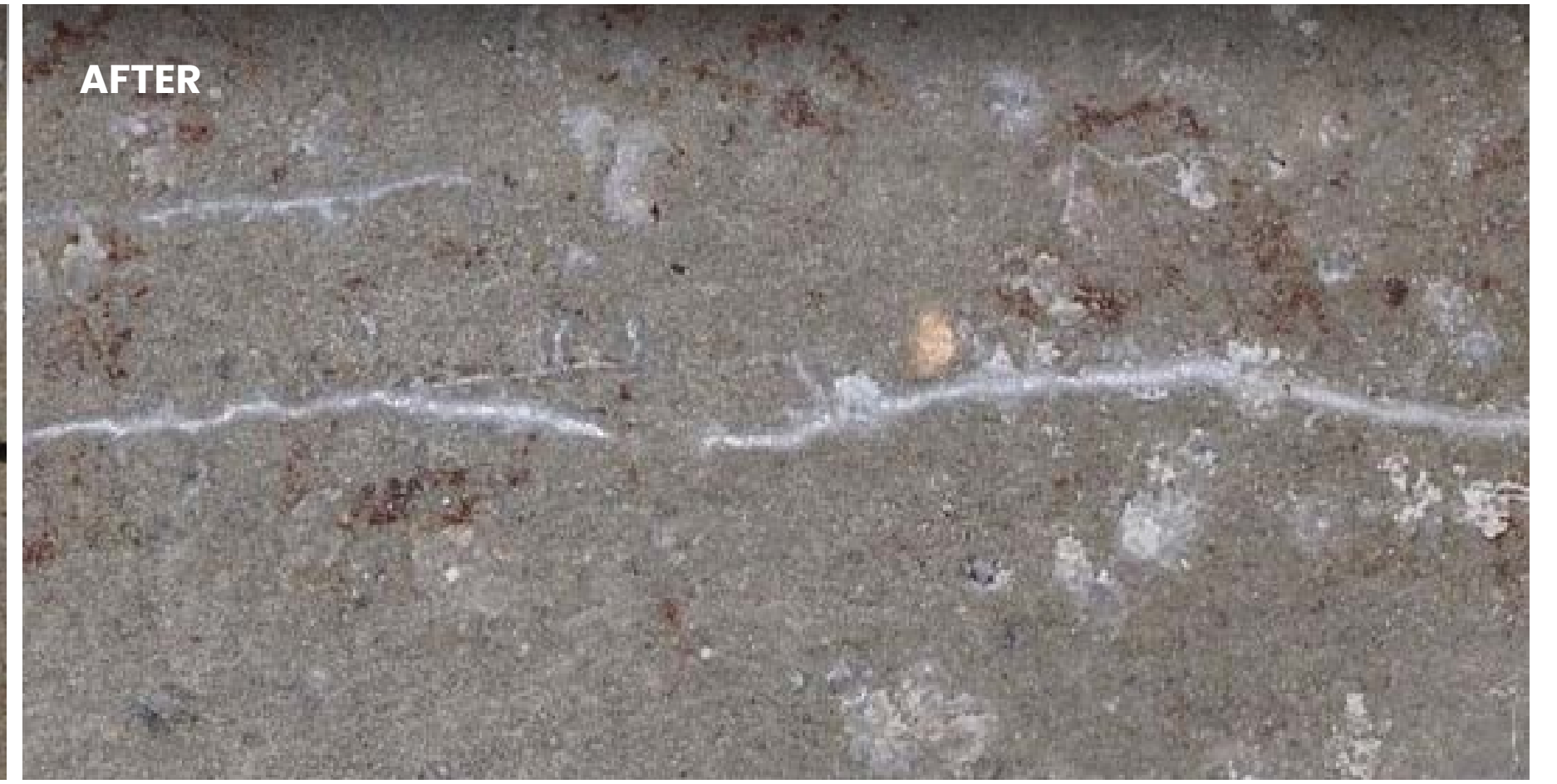
Photomicrographs of a cement containing InvictaSet show a crack before brine exposure (left) is fully sealed after brine exposure thanks to crystalline growth (right).
