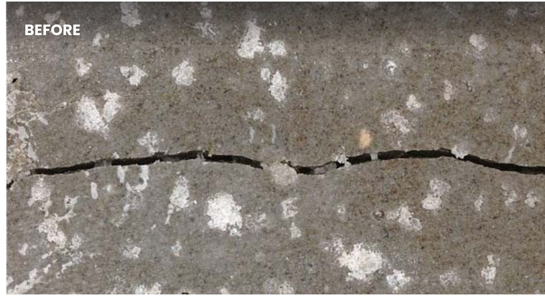
Photomicrographs of a cement containing InvictaSet show a crack before brine exposure (left) is fully sealed after brine exposure thanks to crystalline growth (right).
