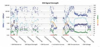
NaviTrak<sup>™</sup> UT maintained high signal strength (3.55 mV) at planned target depth (10,303 ft) to allow drilling to continue. The tool was still decoding at 1.54 mV at final TD of 11,350 ft.
