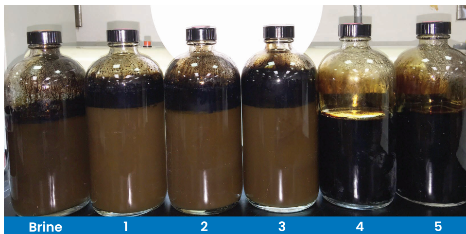
Desalter profile prior to XERIC 7021 treatment
