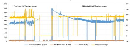
CENesis PHASE performance in a well with high gas content in the fluid stream.
