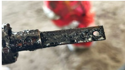
Wax coupon (2-month check) after implementing FORSA PAO3200 was significantly cleaner.
