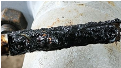
Wax coupon (2 month check) before implementing FORSA PAO3200 showed significant buildup.
