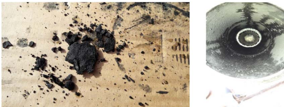
Figure 9—Recovered Debris from VJB
