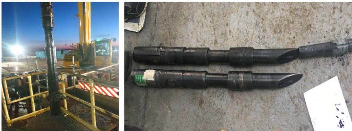
Figure 21—Run 7 Diverter Retrieval & comparison with part of ITTCR on
