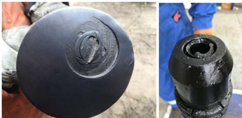
Figure 11—Run 3. LIB result & parted ITTCR retrieved in run 4, removed from overshot at shop
