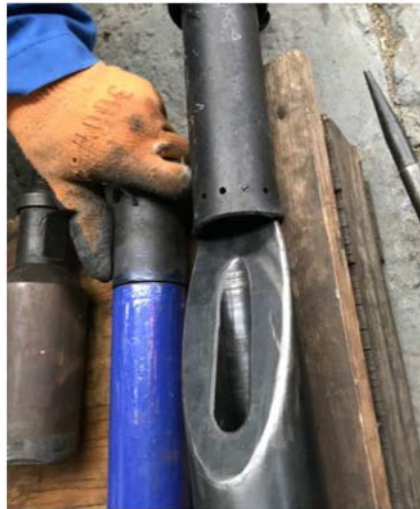
Figure 14—Simulation of how it is believed the parted ITTCR was located above diverter
