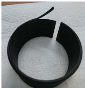
Figure 18—Run 5 broken slip from overshot
