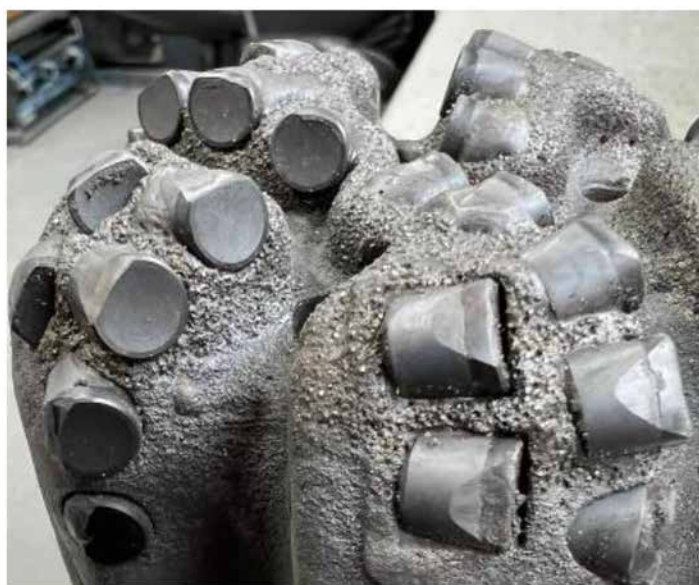
Figure 8—Multi-dimensional non-planar post-run wear state T3
