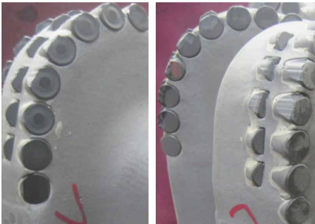
Figure 2—Non-planar (left) vs planar PDC (right) cutter dulls for the same bit frame
