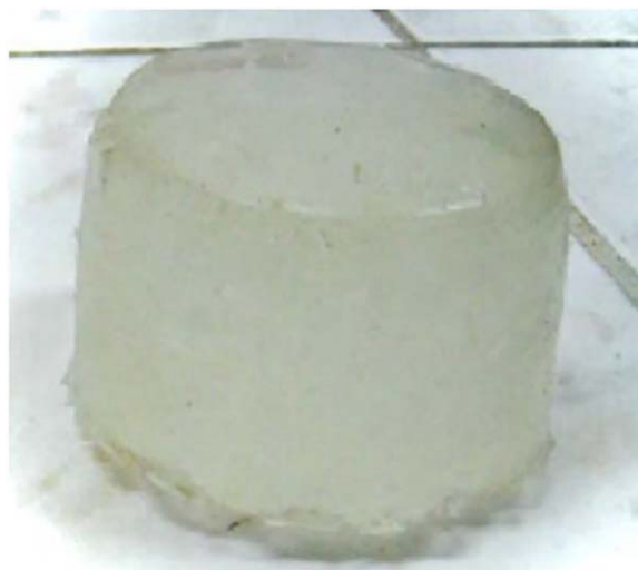
Fig. 6—Solid gel after 7 days at 62°C.
