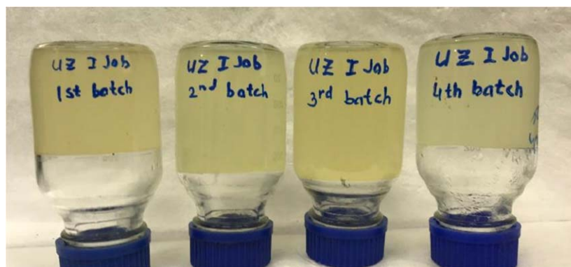
Fig. 9—Crosslinked GSO gel system after 24 hours at 62°C.
