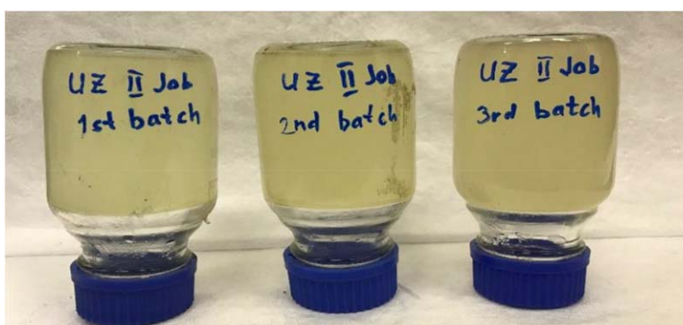
Fig. 11—Crosslinked GSO gel system after 36 hours at 58°C.
