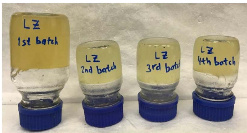
Fig. 16—Crosslinked GSO gel system after 36 hours at 58°C.
