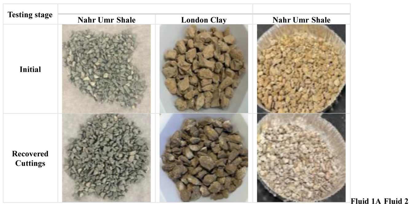
Figure 1—Fluid 1A and Fluid 2: Shale-particle disintegration test results using Nahr Umr shale and London clay.
