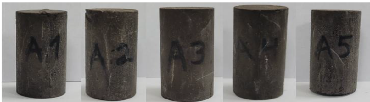
Figure 6—System A – After 6-months in carbonic acid.
