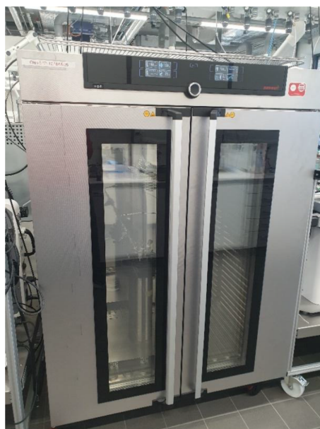
Figure 2—Autoclave inside heating chamber used at the TSC for exposure of cement plugs to CO 2 -saturated formation brine.
