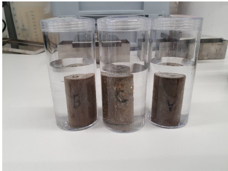
Figure 1—Curing chamber used for CO 2 aging (left) and exemplary photograph of cement plug samples (right).
