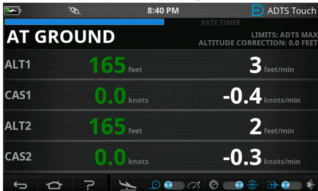
Figura 3-27: Complete Go To Ground – Multicanal
