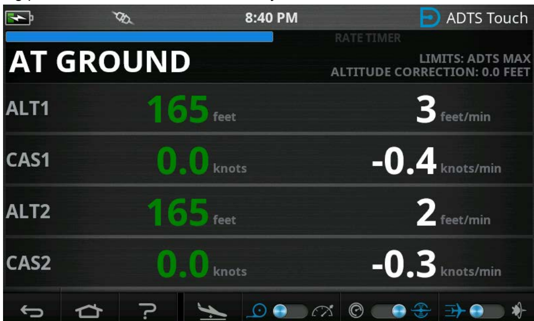
Figure 3-27: Go To Ground Complete – Multi Channel
