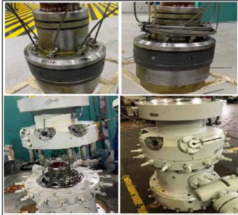
Figure 10—Tubing Hanger System Integration Test
