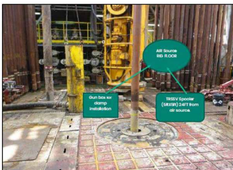
Figure 5—Rig Deck Lay Out
