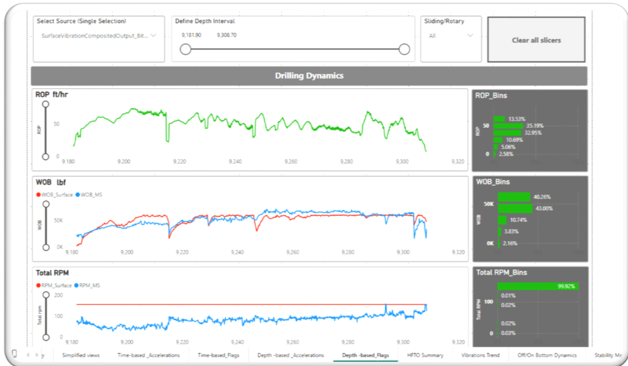
Figure 15—Side-by-side comparison of surface and downhole data.
