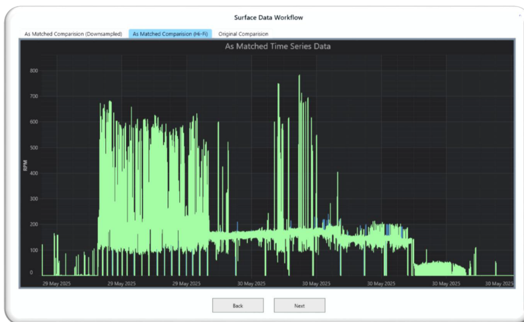
Figure 12—Time shift algorithm matching the surface RPM with downhole RPM.
