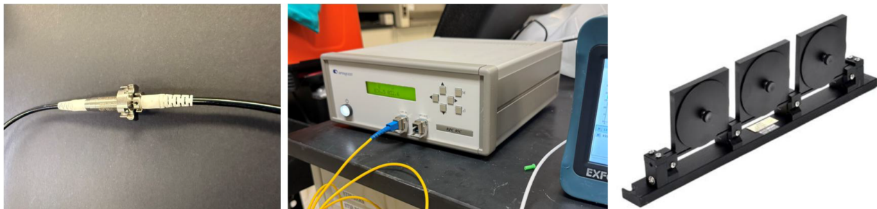
Figure 11—Devices used for polarization sensitivity testing. From left to right: a FORJ unit, a programmable motorized polarization controller, and a 3-paddle manual polarization controller. These devices are used to systematically alter the SOP of the light signal to test the interrogator's performance under dynamic polarization and loss conditions.
