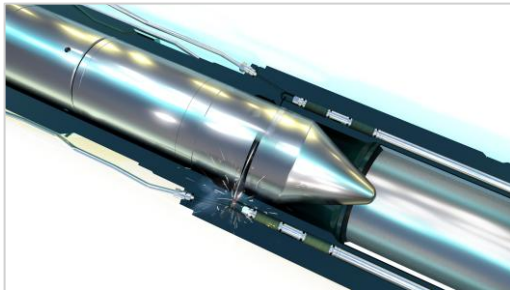
MPC creating hydraulic communication path
